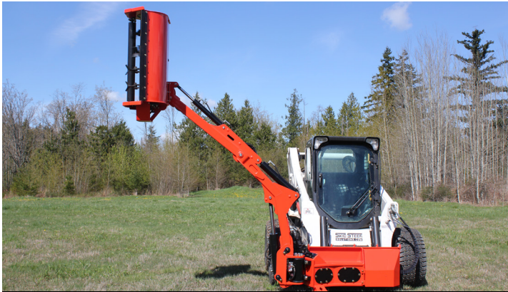
High Mowing Position - Do not transport
