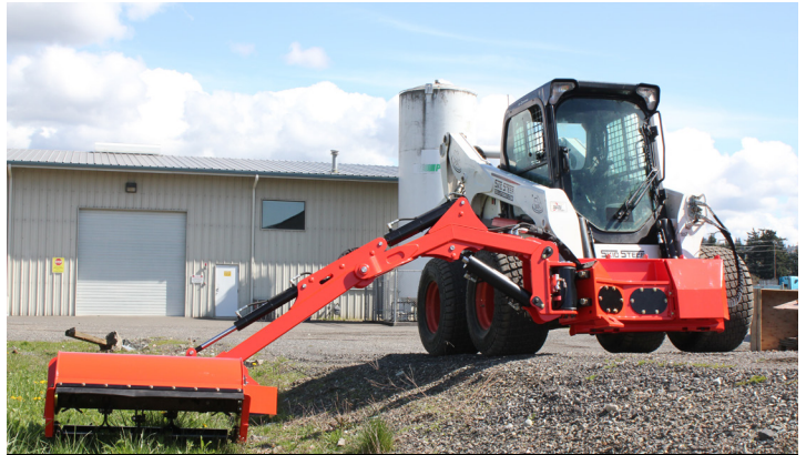
Low Bank Mowing Position - Do not transport
